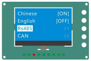
② Select the protocol type you want to set, such as "RS485", and press "ENTER" to enter the RS485 protocol selection page. As shown in the figure below, select the desired protocol name and press "ENTER" to switch "ON/OFF". Select "ON" to successfully set.
